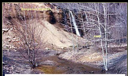
Photo #2 – Dangerous Highwall/AMD – Before Reclamation
