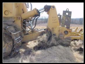
Tractor ripping compacted ground on reclaimed mine site
