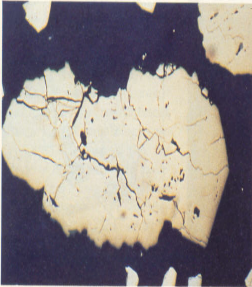
Pyrite particle before biooxidation with bacteria.
